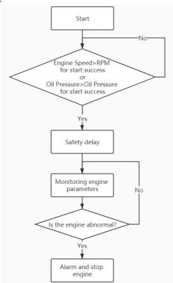
Note: within the safety delay time, only the overspeed alarm will be responded, and other alarms will not respond.
