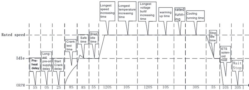
After the manual start is successful, pressing the "automatic key"
